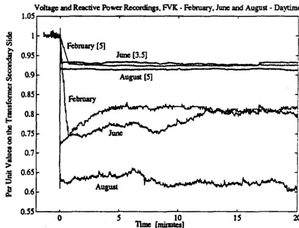
Figure 4.5b. Voltage and reactive power recordings after a voltage reduction in FVK
