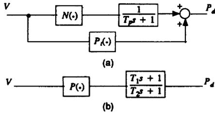
Figure 2.5 Block Diagram Representations of First-order Load Model
