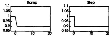
Figure 4.3. Basic shapes of the voltage magnitude variations applied in the two substations; ramp, step
